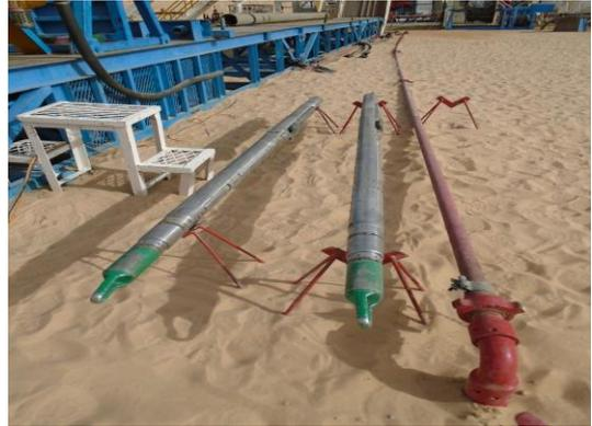
7" liner laid out and ready to run in hole at GW-215.
